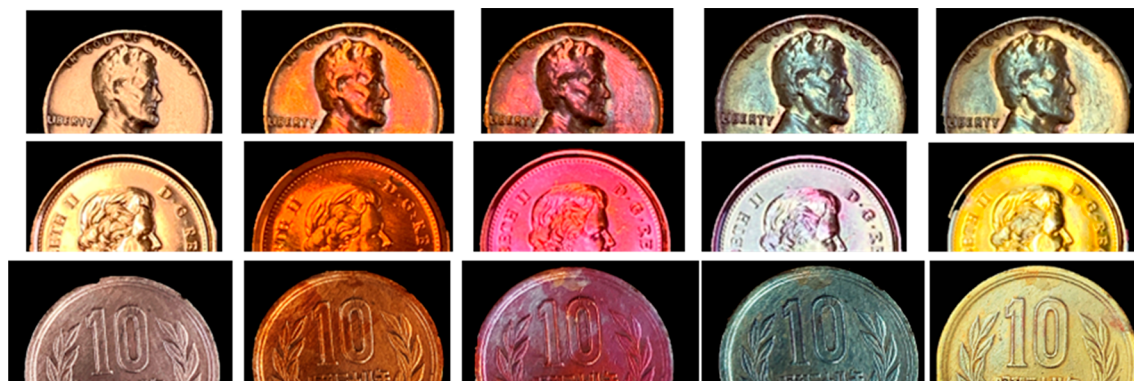
Figure 2. Color progression observed upon heating (top row) a 1968 U.S. penny at 220 °C, (middle row) a 2012 Canadian steel penny at 240 °C, and (bottom row) a Japanese 10-yen coin at 230 °C. The Canadian penny was not buffed with steel wool prior to heating. Increased time heated is from left to right. For appropriate comparison, backgrounds have been blacked out. Pictures of all coins in the last row were taken after quenching in water and placing coins on a lab bench. All other pictures were taken while coins were on a hot plate. All pictures were taken under room lights.
