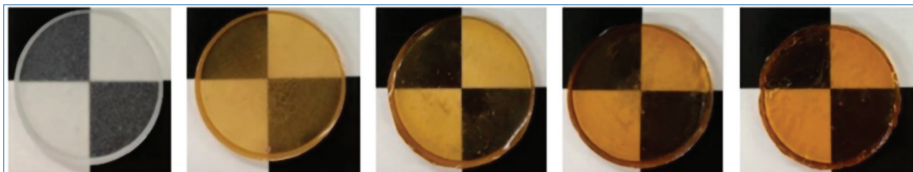
Fig. 2 - Developed DA-containing formulations with progressively increasing DA concentration and bio-based content from left to right
