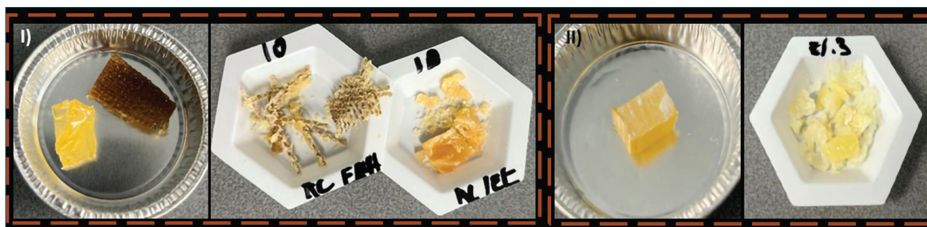
Fig. 5 - WR (I) and ICSO (II) resins and/or composites before and after scCO_2 treatment
