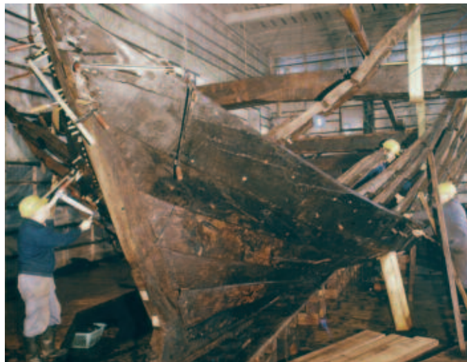
Fig. 4 - The 4 th strake. Reconstructing the cog from waterlogged timbers called for 100% relative humidity - fog - in the cog hall and for constant spraying of the wood. Wooden dowels and treenails proved to be the best choice for assembling the wet timbers (Photo: G. Meierdierks, DSM)
