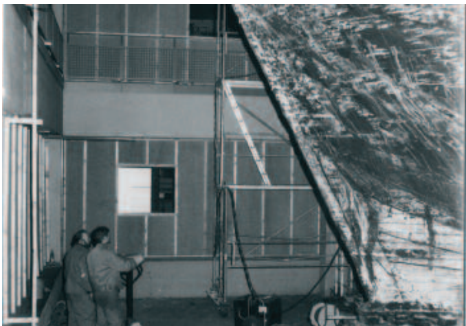
Fig. 9 - Due to the slow pumping-off, the concentrated PEG 3000 solution has solidified on the timbers of the hull (Photo: E. Laska, DSM)
