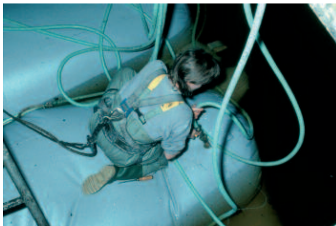
Fig. 6 - Filling displacement balloons in the tank with brine in a tropical climate. The PEG solution had to be kept at 40 °C (Photo: P. Hoffmann, DSM)
