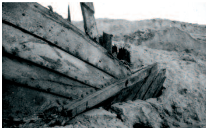
Fig. 2 - A strange hull in the river Weser: very wide clinker-laid planks fastened to each other with big, clenched iron nails run into straight stem posts fore and aft. These are features of a cog (Photo: K. Schierholz, Focke-Museum)
