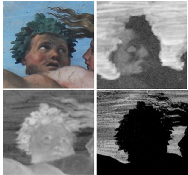
Fig. 2 Detail of triton's head. Top left: visible light image; top right: MA-XRF-map of Cu (Cu is indicated in white); bottom right: RIL image showing Egyptian blue distribution in white; bottom left: MA-XRF-map of Fe (Fe is indicated in white)
