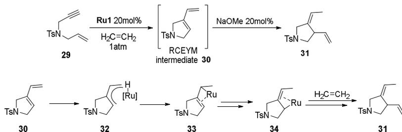
**Scheme 5.** Snapper's tandem RCEYM-hydrovinylation approach.
