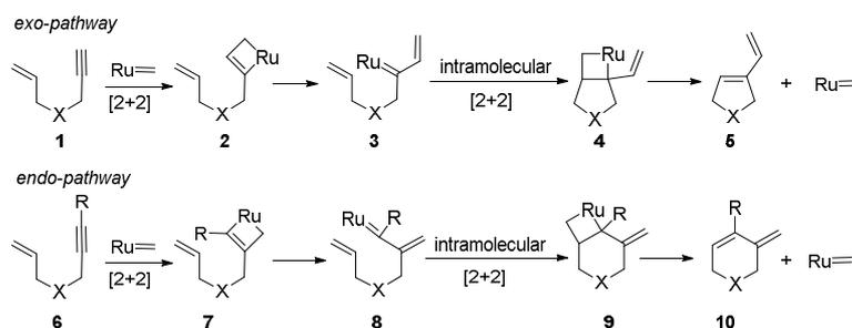
**Scheme 1.** Mechanism of enyne metathesis reaction. *exo*- and *endo*-pathways.
