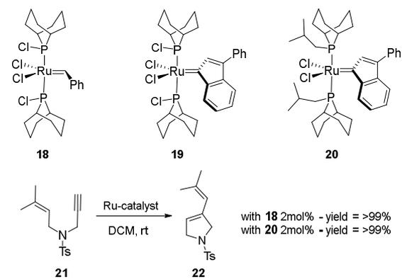
**Scheme 3.** Structures of Phoban-containing pre-catalysts **18-20** and RCEYM
