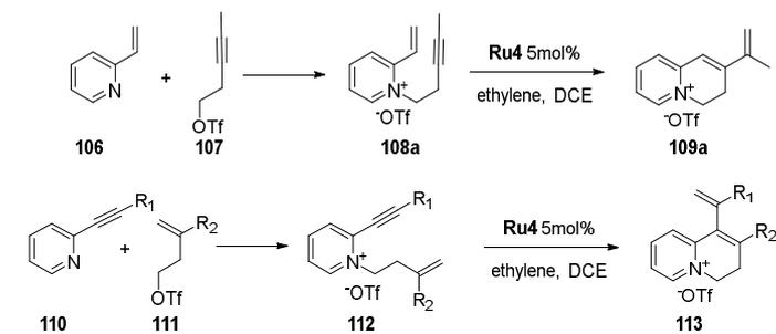
**Scheme 18.** Synthesis of 3,4-dihydroquinolizinium triflates via RCEYM.
