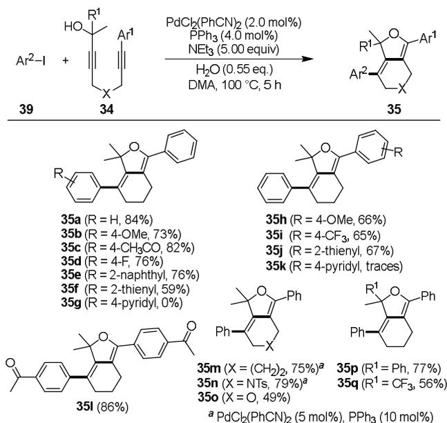
**Scheme 11.** Optimized conditions and products obtained with the *anti*-carbopalladation/*syn*-carbopalladation cascade.
