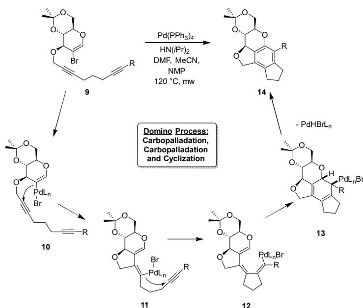
**Scheme 3.** Proposed mechanism of the carbopalladation cascade to yield chromans.
